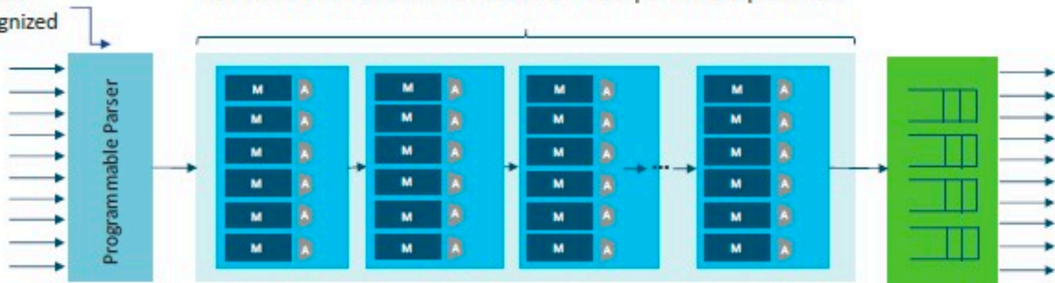
Programmable Pipeline: all stages identical, customer-defined match-action logic
