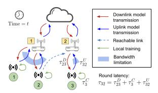
Figure 2: An example of hierarchical FL deployment.
