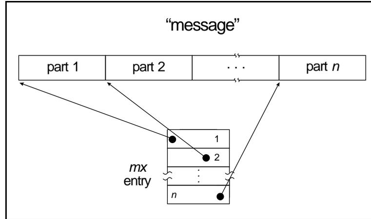
Figure 3. Multi-part messages can be specified with an MX control structure. The microkernel assembles these into a single data stream.
