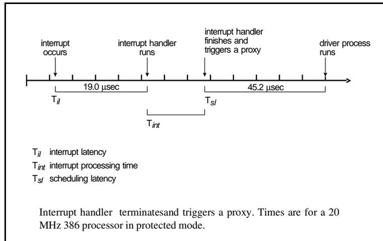
The interrupt latency ( $T_{il}$ ) in the above diagram represents the minimum latency—that which occurs when interrupts were fully enabled at the time the interrupt occurred. Worst-case interrupt latency will be this time plus the longest time in which QNX, or the running QNX process, disables CPU interrupts.
