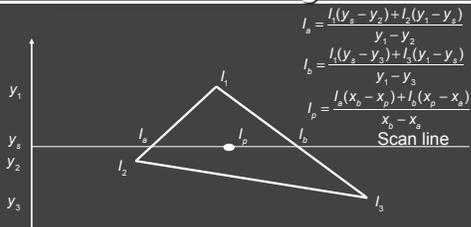
Actual implementation efficient: difference equations while scan converting
