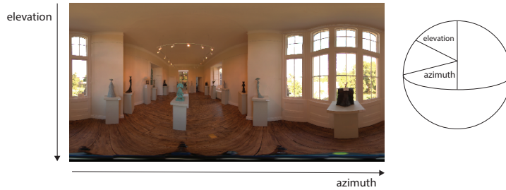
Figure 9: An environment map is an infinitely far away area light that maps each point on a sphere to a directional light source. (Sorry for the abstract drawing. Hopefully you get the idea.)
