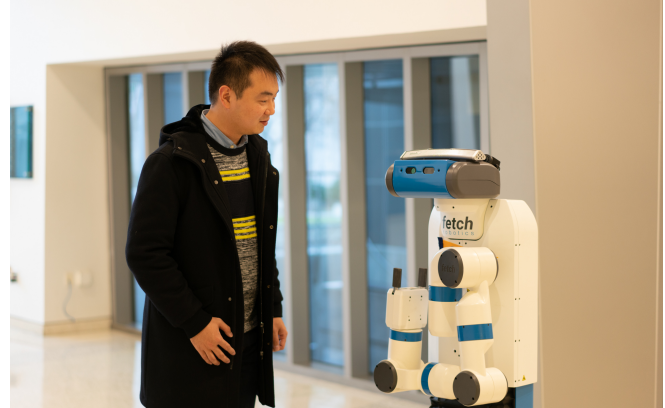
Fig. 1. TritonBot [3]: a Rorg-powered long-term autonomous tour guide robot that chats with people and navigates to introduce places of interest in a university office building. We use Rorg to manage the 41 software components in TritonBot. Rorg only runs the components that are needed and shuts them down when they are idle to save computing resources.
