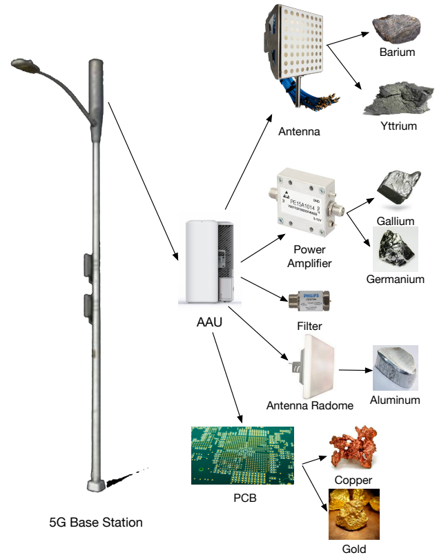
Fig. 1. 5G base station components and materials
