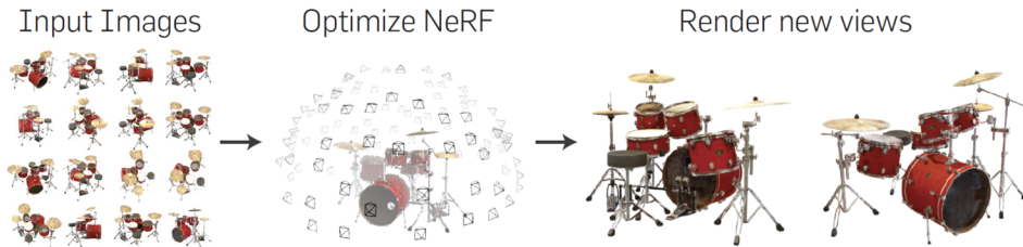
FIGURE 1. The canonical view synthesis problem. Given a set of input images (here 100 views of the synthetic drums scene randomly captured on the surrounding hemisphere), we first optimize a NeRF representation, then use it with volume rendering to synthesize two novel views, including view-dependent specular effects and reflections. For the past three decades, a quest in view synthesis or image-based rendering has been to find the “best” intermediate representation for 3D scenes that will enable the highest-quality view synthesis; this figure could generically represent many previous papers in the area.
