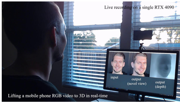
Fig. 14. Our system applied to create a 3D telepresence live from a monocular RGB input. Please see the supplement video for the live demonstration.
