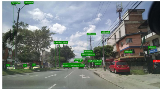
Figure 12. Visualization of the detection results under different methods. We treat a box prediction as true positive if it has an IoU larger than 0.5 with the ground-truth box. The true positive predictions are in green color, while the false positive predictions are in red color. Top-left: Semi-supervised Learning (Semi-SL) method, i.e., Unbiased Teacher-v1 [5]. Top-right: Open-vocabulary object detection (OVOD) method, i.e., OWL-v2 [11]. Bottom-left: AIDE. Bottom-right: ground-truth. Note that some original annotations in Mapillary are not correct. For instance, for the image of “GT” in the second row, the human on the bicycle should be labeled as “bicyclist” while the original label is “person”.
