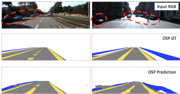
Figure 9. Input image, generated ground-truth pixel-level semantics and predicted semantics from top to bottom row. Our model is able to predict the semantics quite well despite occlusions.
