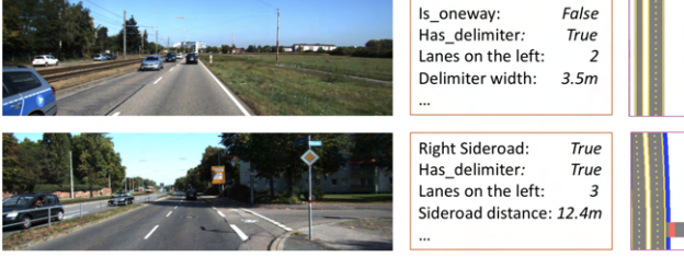
Figure 5. Examples of rendered ground-truth for TS module. From left to right: RGB, parametric human annotations and rendered pixel-level semantics in top-view.
