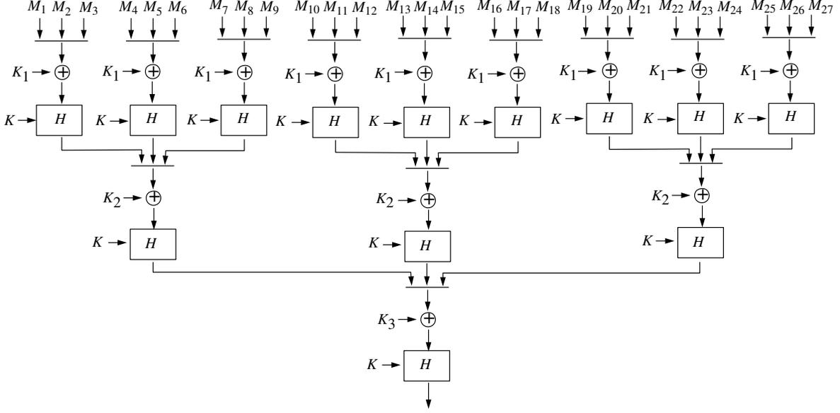
Figure 6: Construction  $XTH$  — The XOR tree scheme, illustrated for  $m = 3$  and  $d = 3$ . Notice that  $H$  is always keyed with  $K$ , while an auxiliary key, differing for each level, is XORed just before the application of  $H_K$ .
