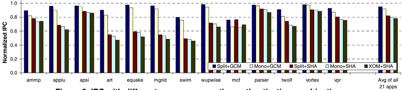
Figure 9. IPC with different memory encryption-authentication combinations.
