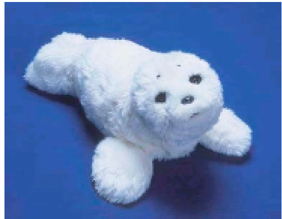
Fig. 2. The PARO robotic seal robot. This robot is embodied within a stuffed animal, and acts as one might expect an animate toy to behave. It has generally been well accepted as a companion robot. Photograph © 2005 ACM.
