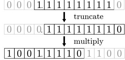
Figure 10: Worst-case error example when generating digits. The dark boxes correspond to an 8-bit floating-point number with a leading 1 bit. Grey boxes correspond to bits that the number cannot represent. Notice that they are grey after the multiplication, indicating that they are lost due to truncation.
