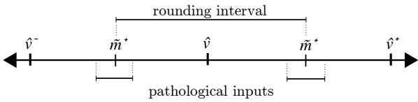
Figure 12: Pathological Input Range. Pathological inputs occur in a small area immediately surrounding the midpoints  $\tilde{m}^-$  and  $\tilde{m}^+$ .
