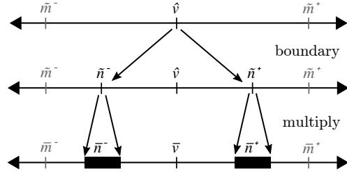
Figure 3: Error Propagation. The *multiply* operation computes the scaled interval  $(\bar{n}^-, \bar{n}^+)$  with error (as represented by the black boxes), creating the requirement that the narrow interval  $(\tilde{n}^-, \tilde{n}^+)$  be conservative enough to prevent overlap with the scaled midpoints  $\tilde{m}^-$  and  $\tilde{m}^+$ .
