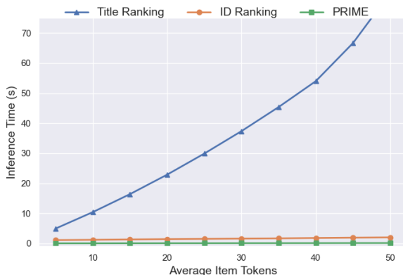
Figure 7: Inference efficiency of PRIME compared to list-wise generation of item titles and IDs. X-axis represents average item token length and y-axis represents inference time.
