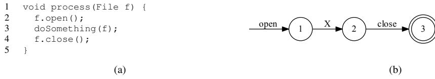
Fig. 1 (a) Simple code snippet using File . The methods open and close are API methods, and the method doSomething is unknown. (b) Symbolic automaton mined from this snippet. The transition corresponding to doSomething is represented using the variable X . Transitions corresponding to API methods are labeled with method name.
