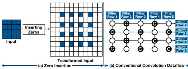
Figure 4: (a) Zero-insertion step in a transposed convolution operation for a  $4 \times 4$  input and the transformed input. The light-colored squares display zero values in the transformed input. (b) Using conventional dataflow for performing a transposed convolution operation.
