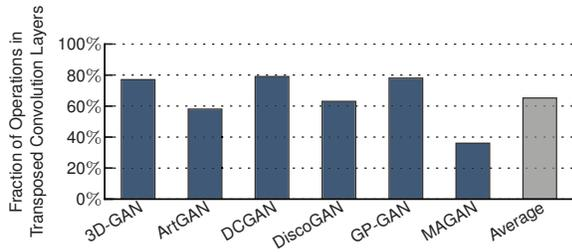
Figure 1: The fraction of multiply-add operations in transposed convolution layers that are inconsequential due to the inserted zeros in the inputs.
