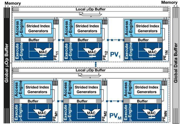
Figure 6: Top-level block diagram of GANAX architecture.
