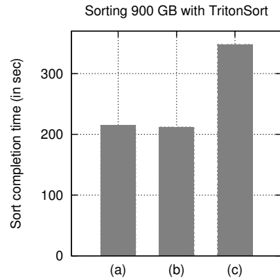
Figure 3: TritonSort completion time in three cases: (a) Fully non-blocking electrical switch (baseline case) (b) Helios/c-Through network with no background flows (c) Helios/c-Through network with one competing background flow
