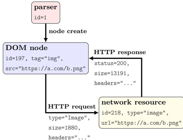
**Fig. 4.** PageGraph encoding of the initialization of an image element. The browser’s HTML parser creates a DOM node to represent a decoded `<img>` tag. An HTTP request is dispatched to retrieve the image file pointed to by the image element’s `src` attribute, and a success response is received.
