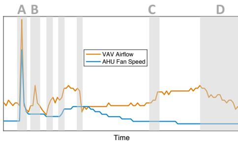
**Figure 2: Example sensor readings from a VAV and its connected AHU. The VAV events (in grey) have many different causes—it can result from a change in the AHU (coincident event A) or changes in the served space (unique event B,C,D). Only the coincident ones help identify the functional connection between equipment.**
