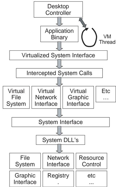
**Figure 3: Shows the virtual layer placed between the application binary and dlls and the operating system. In addition, a VM Portal (VM thread) is started in the application to maintain a lifeline to the Desktop Controller.**
