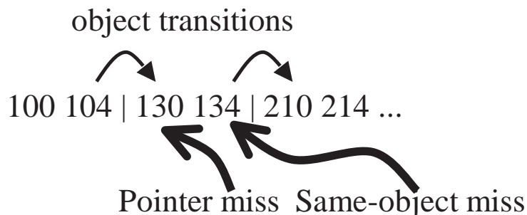
Figure II.5: Potential miss stream depicting Same Object and Pointer misses corresponding to linked data structure accesses. Object boundaries are depicted with vertical bars and transitions are marked by arrows. The first miss following a transition is classified as a Pointer miss while misses to different fields of the same object are classified as Same-Object misses.
