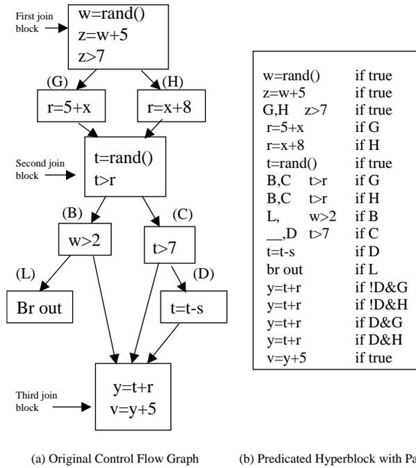
Figure 2: Code is duplicated when more than one definition reaches a use to maintain maximum flexibility for the scheduler. In (b), the statement  $y=t+r$  is duplicated for each pair of definitions that may reach this statement. Each copy is guarded by the predicates that defined the path along which those definitions would occur.
