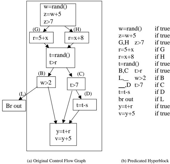
Figure 4: Extended example of transformation from non-predicated CFG to predicated hyperblock
