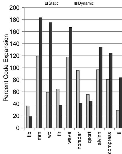
Figure 13: Static and Dynamic Code Expansion normalized to original code size. Dynamic code expansion indicates an increase in the working set size to be supported by the instruction cache.
