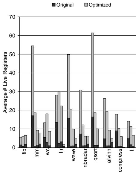
Figure 12: Weighted average register pressure in hyperblocks when using PSSA with Predicated Speculation and Control Height Reduction. Shown from left to right for each benchmark is the general purpose file, predicate file, branch file, and floating point file (zero utilization for some benchmarks).
