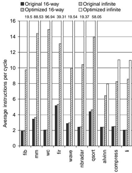
Figure 11: Weighted average number of operations scheduled per cycle for hyperblocks when using PSSA with Predicated Speculation and Control Height Reduction. Note that several of the "Optimized infinite" results are greater than 16 – the issue width simulated in these experiments.
