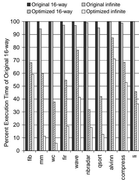
Figure 10: Executed cycles normalized to the number of cycles to execute the original code produced by Trimaran for a 16 issue machine.
