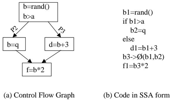
Figure 3: Static Single Assignment
