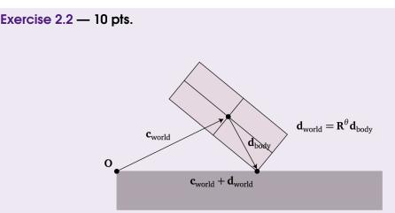
A classic treatment for handling collision in a rigid body simulation is the following. Whenever a vertex of a moving body penetrate another object, "push" the positional variables  $\mathbf{q}$  back to the feasible set and "readjust" the velocity so that the change in the momentum is in the range of the pullback of constraint on the world position.
