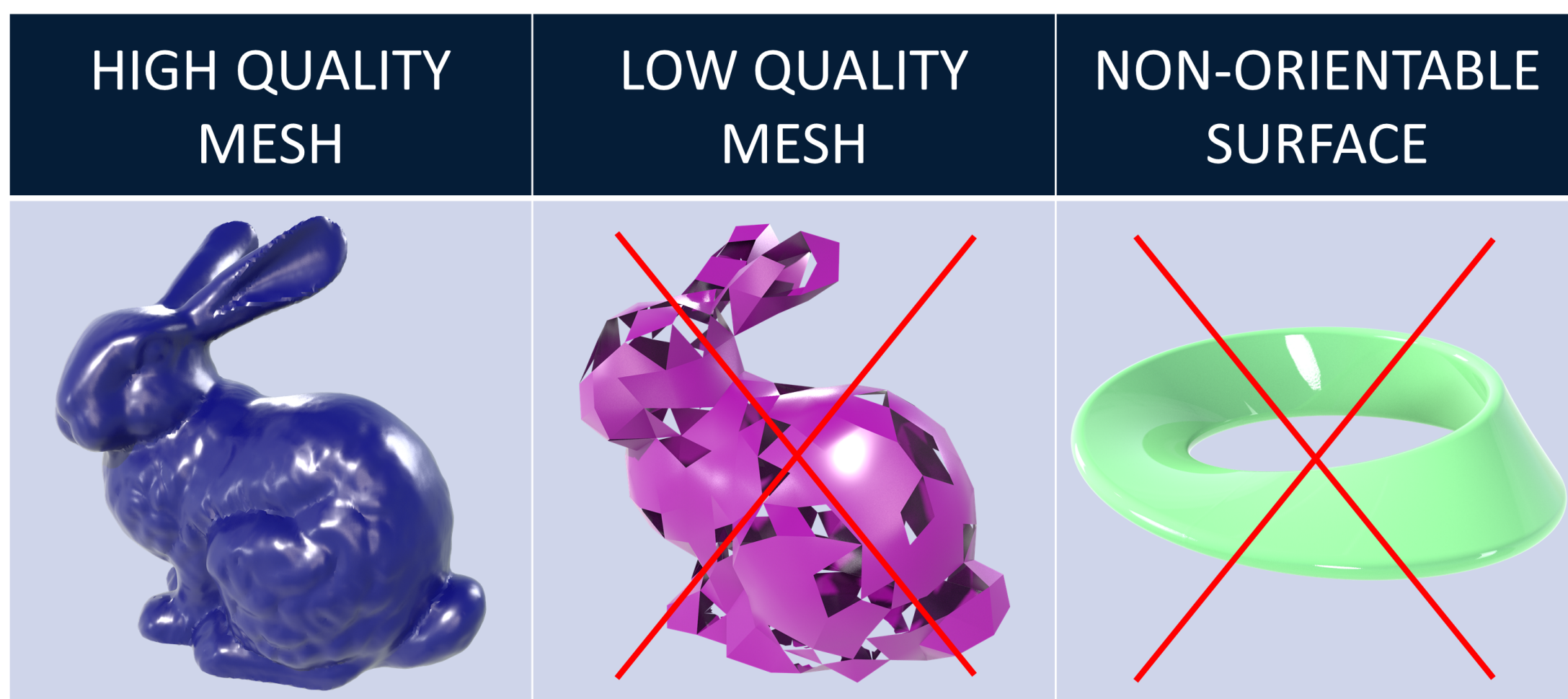
Figure 1: DEC works on high-quality meshes, but fails on low-quality meshes or complex surfaces
