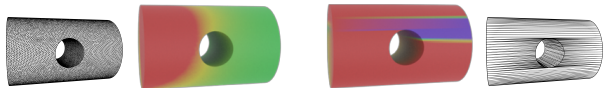
Figure 1: Heat flow simulated with DEC on a high quality mesh (left) and on a poor mesh (right). Wireframe renders of the mesh are shown next to each simulation.
