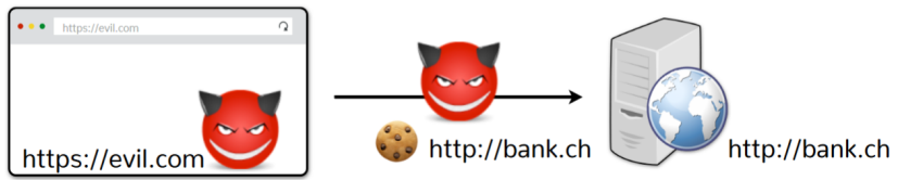
Figure 19: Web attack making cross-origin request
