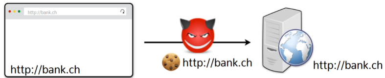
Figure 20: Network attacker stealing cookies on unencrypted HTTP traffic
