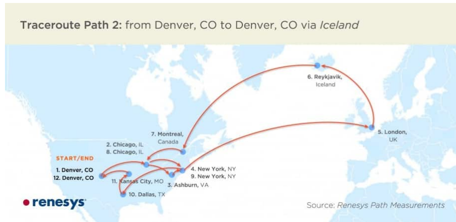
Figure 7: Traffic from Denver, Colorado to Denver being routed through London and Reykjavik, Iceland [2]
