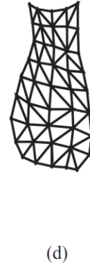
Figure 12.5 Range data scanning (Curless and Levoy 1996) © 1996 ACM: (a) a laser dot on a surface is imaged by a CCD sensor; (b) a laser stripe (sheet) is imaged by the sensor (the deformation of the stripe encodes the distance to the object); (c) the resulting set of 3D points are turned into (d) a triangulated mesh.
