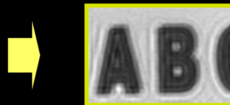
Ringings with the traditional Richardson-Lucy deconvolution algorithm
