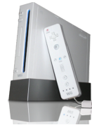
Nintendo Wii has camera-based IR tracking built in.
