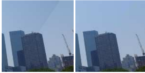
Figure 4: (Left) Zoom-in of seam artifact caused by vignetting. (Right) Result after vignetting correction.
