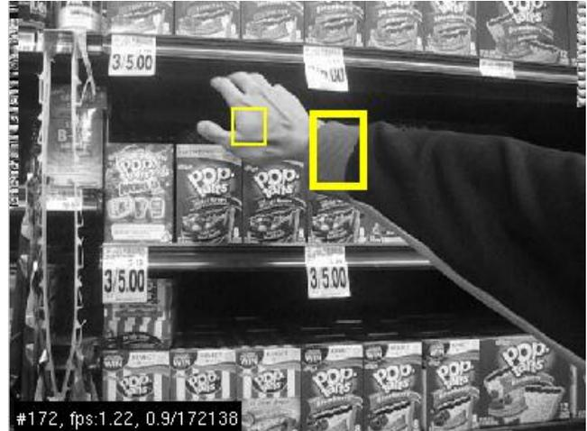
Figure 9. Occluded product mostly visible, but detection is now focused on the jacket cuff due to a new crop of positive examples containing the jacket cuff
