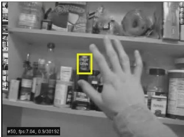
Figure 1. Bounding box around product just before occlusion (negative examples in column along left side, positive examples in column on right side)
