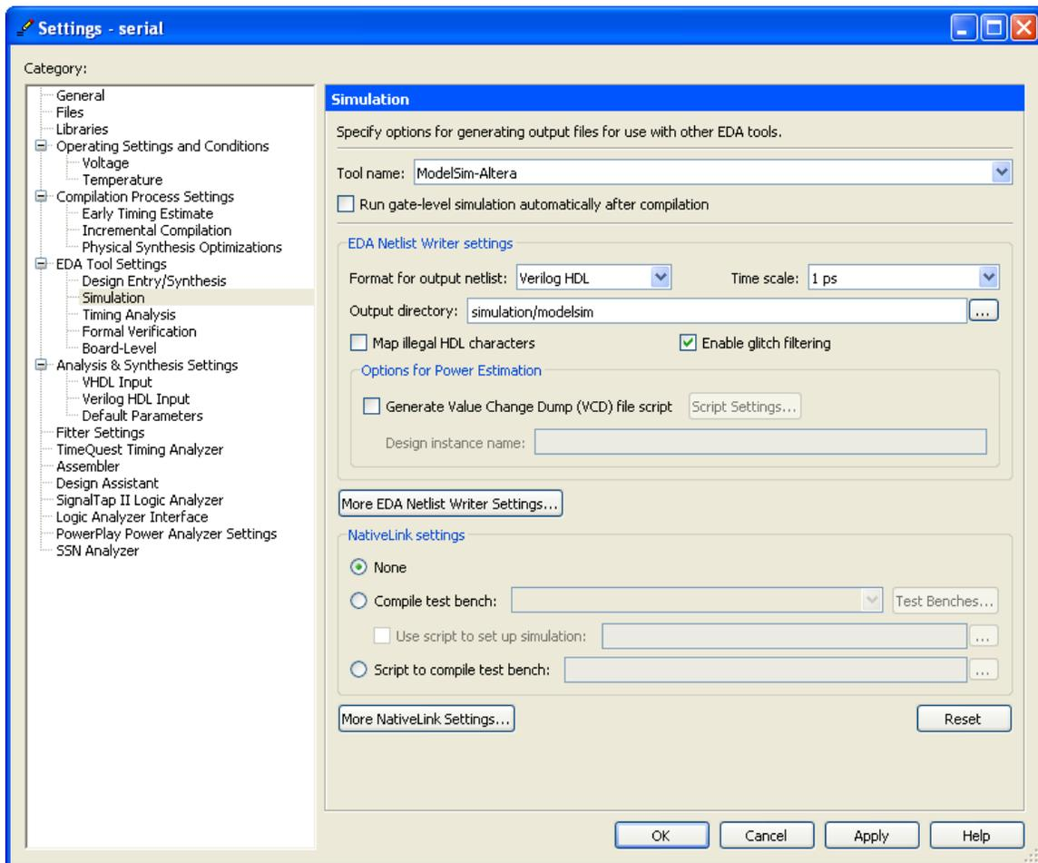
Figure 24. Quartus II EDA simulation tool settings.
