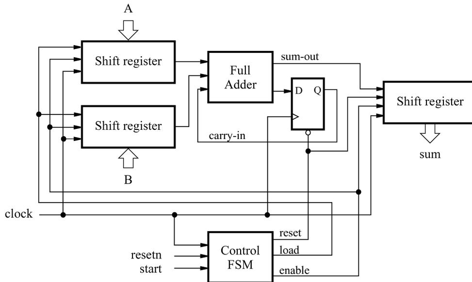
Figure 2. Block diagram of a serial-adder circuit.
