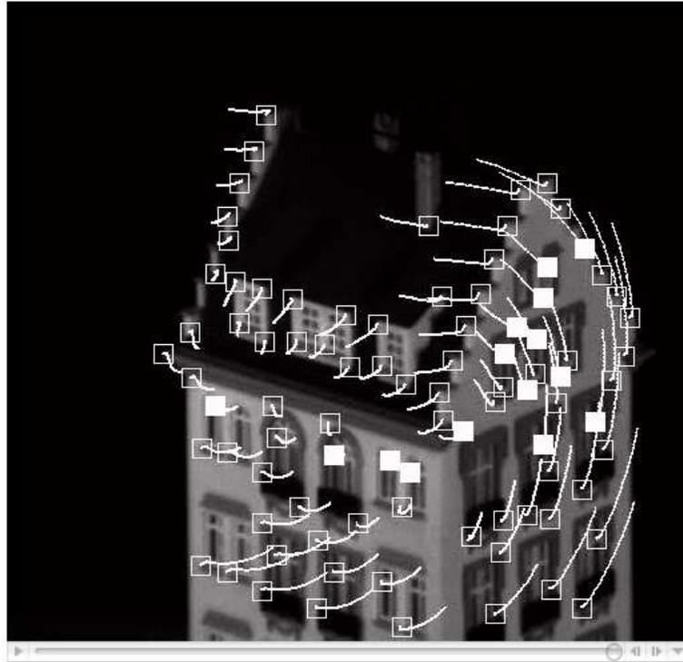
**Figure 6.** This photo shows the tracked movement of image patches of a building over a number of successive frames in a movie. The patches are tracked using an affine model. [Tommasini et al.]
