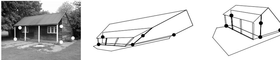
**Figure 3.** Direct upgrade from projective to Euclidean using 5 ground-truth points, which are in general position (i.e., no 4 points are coplanar). (H&Z Figure 9.6).
