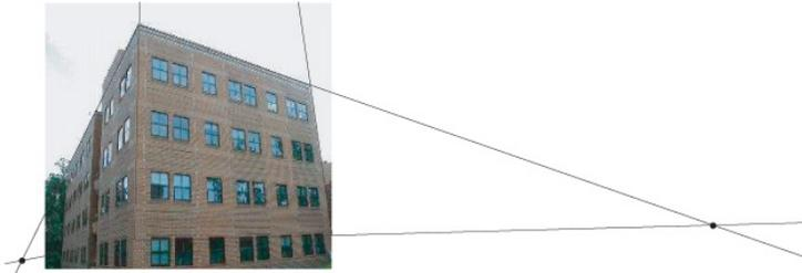
**Figure 2.** Parallel lines and the associated vanishing points. (MaSKS Figure 6.12) Two vanishing points are shown; the third is off the page far above the picture.
