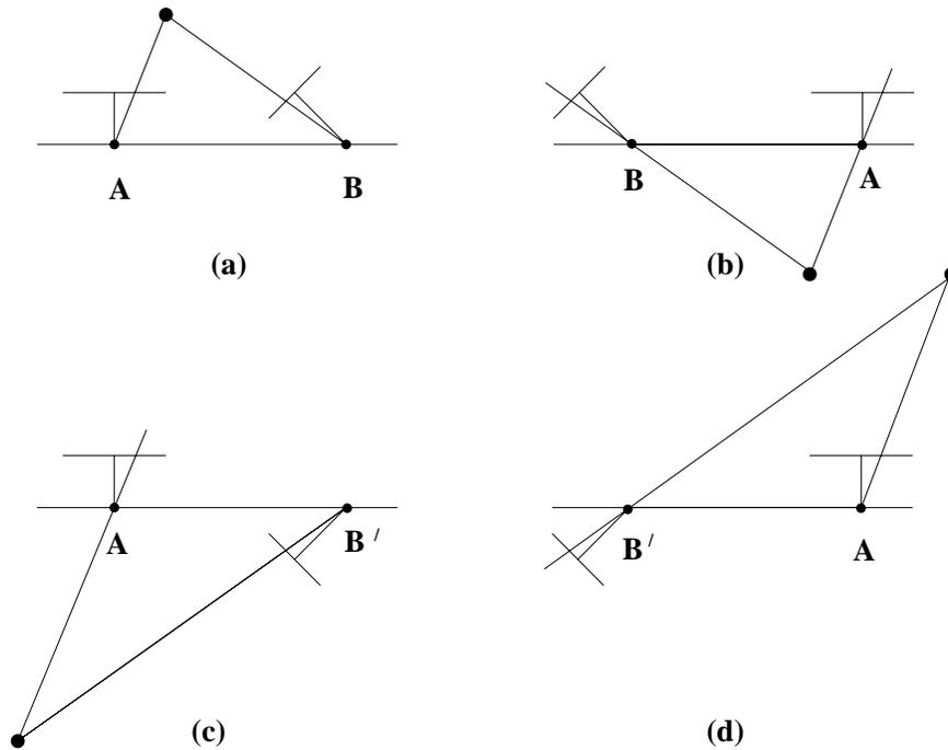
Fig. 8.12. **The four possible solutions for calibrated reconstruction from  $E$ .** Between the left and right sides there is a baseline reversal. Between the top and bottom rows camera  $B$  rotates  $180^\circ$  about the baseline. Note, only in (a) is the reconstructed point in front of both cameras.
