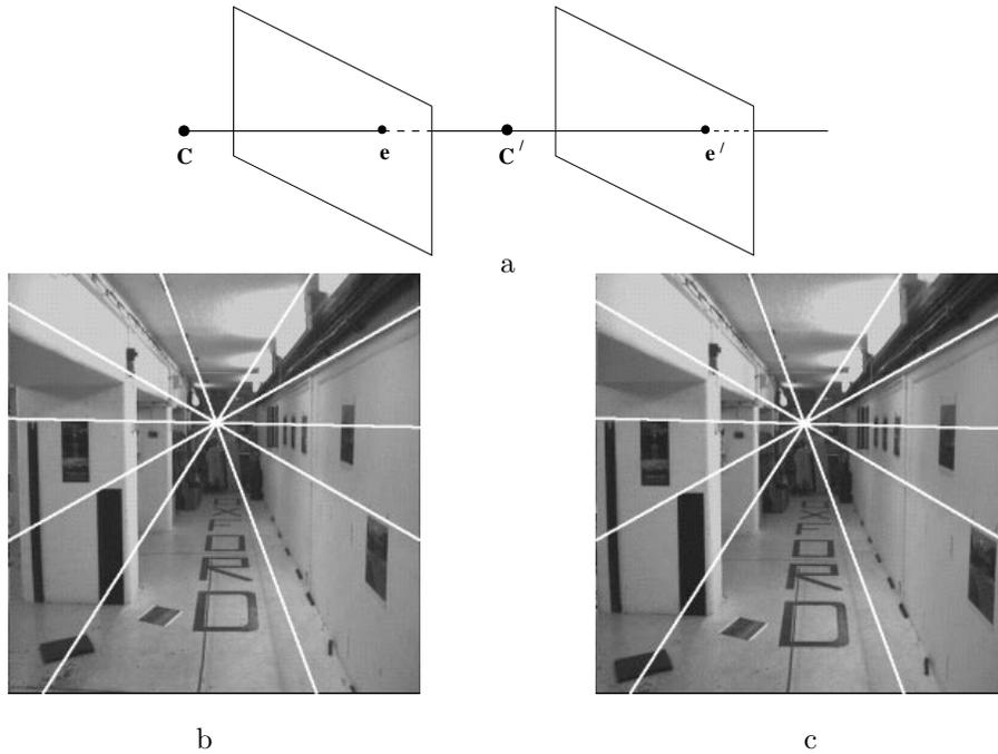
**Fig. 8.8. Pure translational motion.** (a) under the motion the epipole is a fixed point, i.e. has the same coordinates in both images, and points appear to move along lines radiating from the epipole. The epipole in this case is termed the Focus of Expansion (FOE). (b) and (c) the same epipolar lines are overlaid in both cases. Note the motion of the posters on the wall which slide along the epipolar line.
