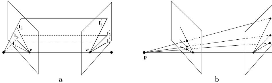
Fig. 8.6. **Epipolar line homography.** (a) There is a pencil of epipolar lines in each image centred on the epipole. The correspondence between epipolar lines,  $\mathbf{l}_i \leftrightarrow \mathbf{l}'_i$ , is defined by the pencil of planes with axis the baseline. (b) The corresponding lines are related by a perspectivity with centre any point  $\mathbf{p}$  on the baseline. It follows that the correspondence between epipolar lines in the pencils is a 1D homography.
