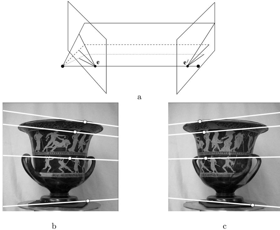
Fig. 8.3. **Converging cameras.** (a) Epipolar geometry for converging cameras. (b) and (c) A pair of images with superimposed corresponding points and their epipolar lines (in white). The motion between the views is a translation and rotation. In each image, the direction of the other camera may be inferred from the intersection of the pencil of epipolar lines. In this case, both epipoles lie outside of the visible image.
