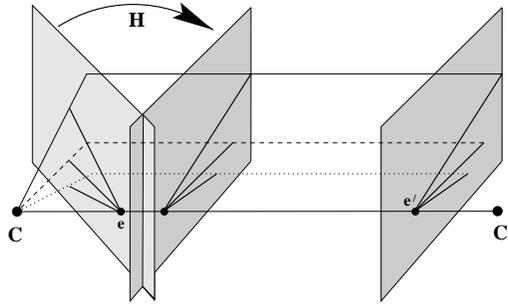
Fig. 8.9. **General camera motion.** The first camera (on the left) may be rotated and corrected to simulate a pure translational motion. The fundamental matrix for the original pair is the product  $\mathbf{F} = [\mathbf{e}']_{\times} \mathbf{H}$ , where  $[\mathbf{e}']_{\times}$  is the fundamental matrix of the translation, and  $\mathbf{H}$  is the projective transformation corresponding to the correction of the first camera.
