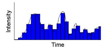
Sampling will take an analog signal (the black line above) and convert into digital representation (the blue bars). Each of these blue bars represents the intensity of the signal at a point in time.
