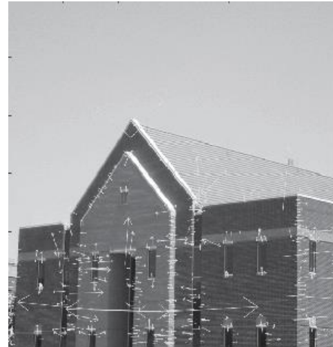
FIGURE 12.61 The keypoints from Fig. 12.60 superimposed on the original image. The arrows indicate keypoint orientations.
