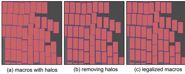
Figure 2: Easing legalization with macro halos. Removing macro halos leaves enough space for macros to be legalized without significantly disrupting the standard cells and other macros.
