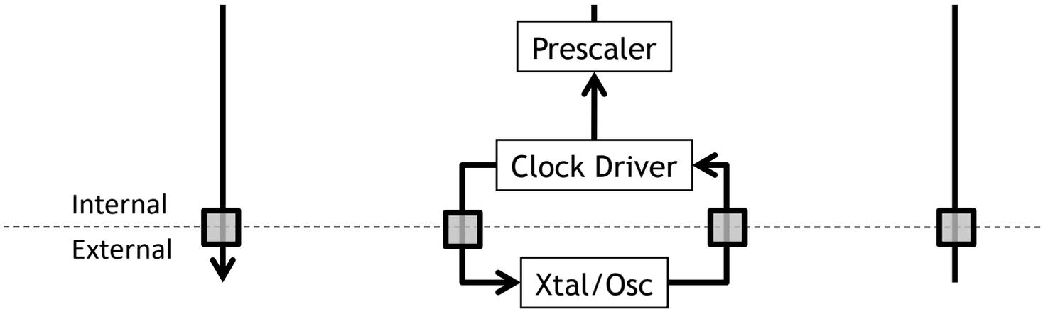
Frequency depends on the attached oscillator device
