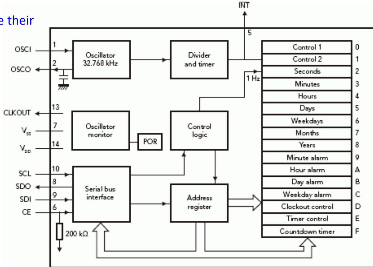
The reason the 32,768 Hz resonator has become so common is due to a compromise between the large physical size of low frequency crystals and the large current drain of high frequency crystals.
