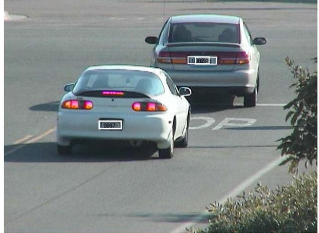
Figure 10: Detected license plate locations on a frame from a live video stream.
