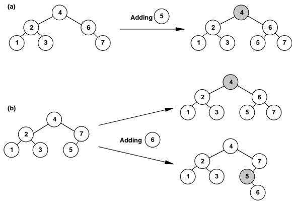
Fig. 23. Adding Prefix Lengths (Gray Nodes change Rope)
