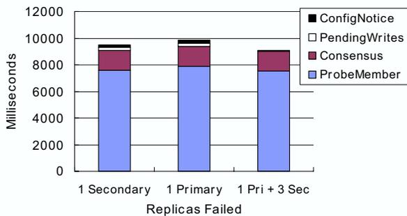
Figure 11: The cost of failure-induced reconfigurations as observed by the primary of the *new* configuration. All experiments start from a five-replica configuration and then we kill a particular set of replicas.
