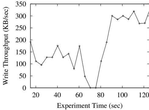
Figure 12: Measured write throughput under regeneration.
