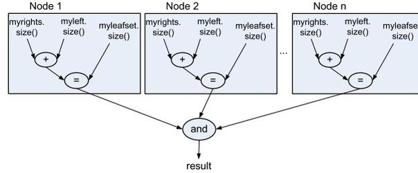
**Fig. 5.** Example of using a dataflow graph to represent the Pastry LeftRight property
