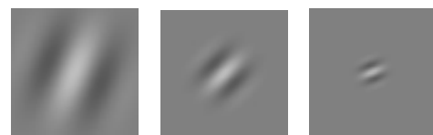
Fig. 4. Real components of Gabor wavelet filters at three different orientations and scales.
