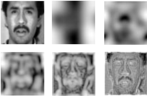
Fig. 5. Original image and Gabor jets at five scales. Each pixel's intensity in the processed images represents the log of the sum of the magnitudes of the filter responses in each of the eight directions.
