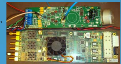
Fig. 5. Prototype hardware for one node. The hardware includes the transducer (ring in upper right corner), the analog circuit (upper board) and an DINI group's DNMEG_ADDA evaluation board. The two boards are connected via SMA cables.
