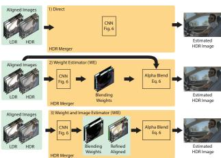
Fig. 5. Each row demonstrates a different architecture for learning the HDR merge process. The top row shows the architecture where we model the entire process using a CNN. We constrain the problem for the other two architectures (middle and bottom rows) by using the knowledge from existing techniques. See the text in Sec. 3.2 for more details.
