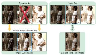
Fig. 7. We ask a subject to stay still and capture three bracketed exposure images on a tripod which are then combined to produce the ground truth image. We also ask the subject to move and capture another set of bracketed exposure images. We construct our input set by taking the low and high exposure images from this dynamic set and the middle exposure image from the static set.
