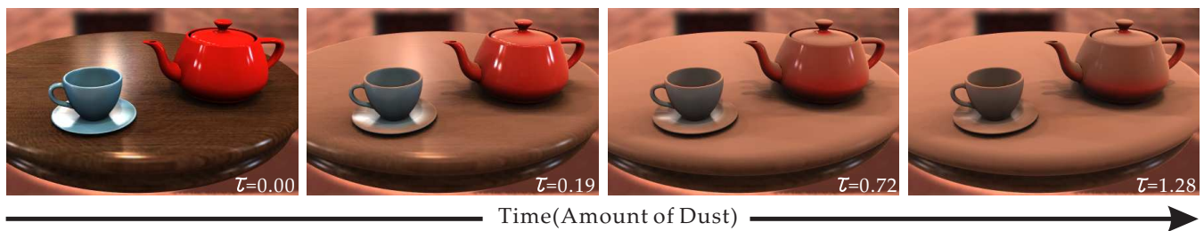
Fig. 1. Rendered images of dust accumulating in a tea set scene, leading to effects such as the diffusing and fading of specular highlights and the shifting of the diffuse component resulting in overall changes in color saturation and hue. The teapot and teacup are rendered with our acquired data, and the table with a novel material showing the same characteristic time-varying behavior. Please refer to Figure 15 for enlarged insets and Section VI for more details.
